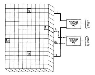
Fig. 1(a)—The photomosiac and two of the randomly chosen photocell pairs. The four digital groups to the right are the four possible states of each photocell pair.
