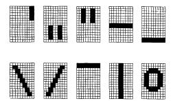
Fig. 9—Arbitrary shapes which were taught to the system as a basic distribution pattern for the subsequent reading of alphanumeric handwritten characters. Each shape was learned in the position shown and also in several positions resulting from lateral displacement.
