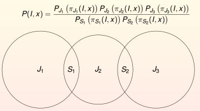
$S_1$  is called a separator of the nodes in  $J_1$  and the nodes in  $J_2$  because if the nodes in  $S_1$  are deleted, what remains of  $J_1$  and  $J_2$  are separated. In fact, if the nodes in  $S_1$  are deleted,  $J_1 - S_1$  and  $(J_2 - S_2) \cup J_3$  are separated.
