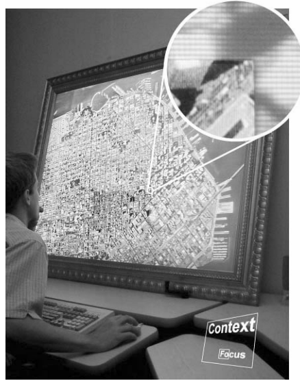
Fig. 13. A mixed-resolution large display using a 1024 \times 768 LCD panel focal area inset within a 1024 \times 768 projected contextual display (with permission of Baudisch et al. [2002]).
